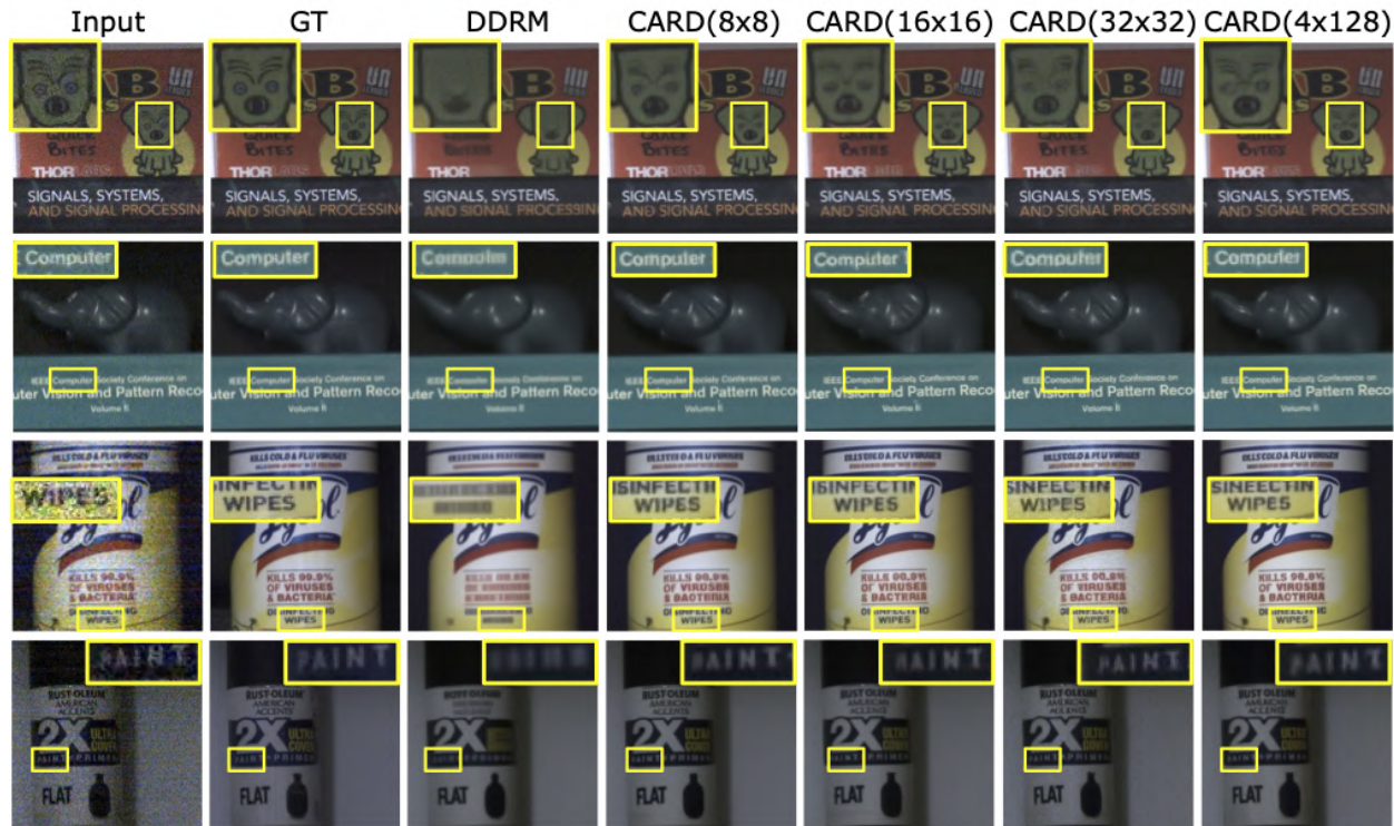
Figure 4. Effect of patch size on CARD denoising quality. Top two rows show low-noise images where smaller patches ( 8 \times 8 , 16 \times 16 ) produce slightly clearer outputs. Bottom two rows show high-noise images where larger and anisotropic patches ( 32 \times 32 , 4 \times 128 ) yield improved visual quality by better capturing spatial noise correlations.
