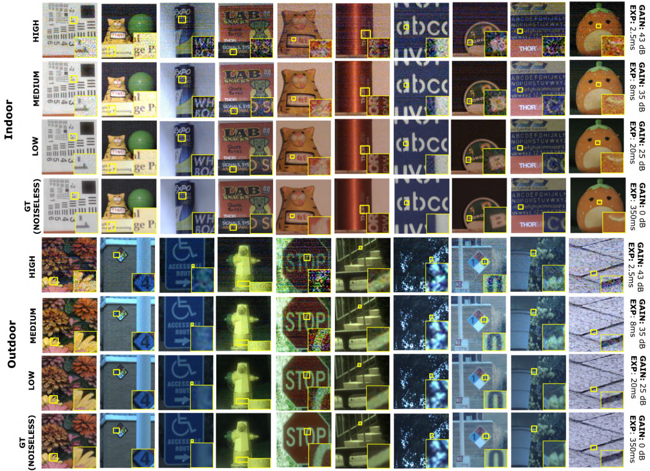
Figure 1. CIN-D dataset examples. CIN-D contains images of the same scenes captured at different noise levels using a FLIR Blackfly S BFS-U3-63S4C-C color camera. Noise levels decrease from top to bottom through controlled variations in sensor gain and exposure time, while scene content and viewing geometry remain fixed. This illustrates the progressive degradation in image quality that our dataset captures for benchmarking restoration algorithms under realistic correlated noise conditions.
